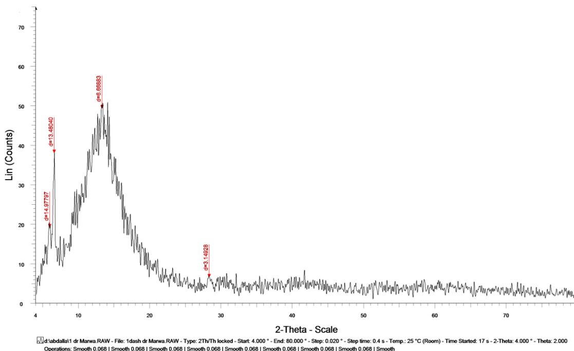
**Fig. 8 : X-Ray diffraction spectrum of Mn-2-ethyl hexanoate crystals**
