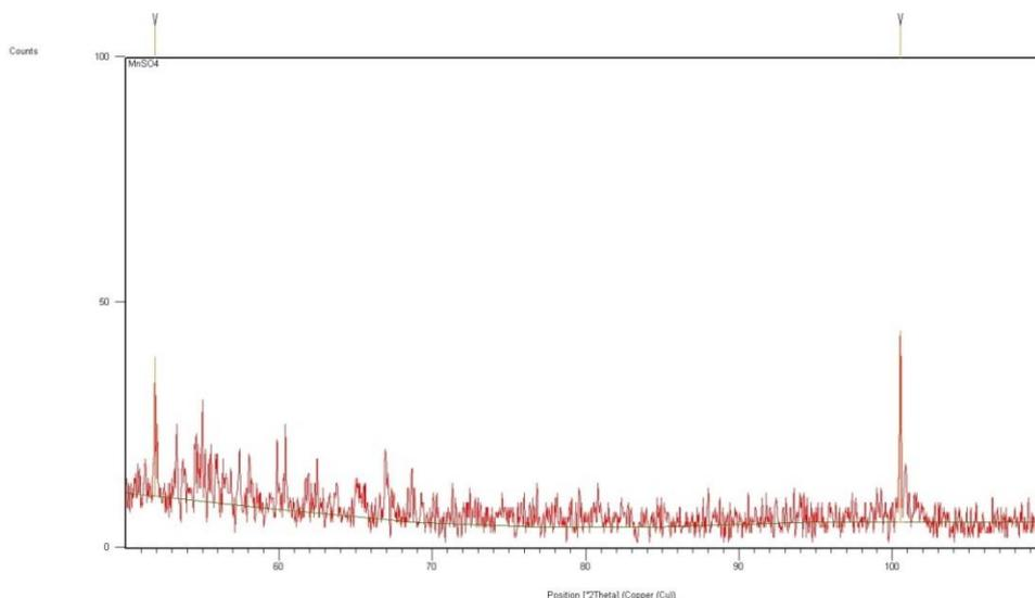
**Fig.6 : X-Ray diffraction pattern of a typical manganese sulfate sample prepared using oxalic acid as reducing agent**
