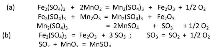
It is possible that under these conditions the dissociation of sulfur trioxide is catalyzed by ferric oxide. Thermal treatment above 640°C decreased considerably the amount of ferric sulfate, but manganous sulfate was stable up to 850°C, and only above 950°C did it decompose to  $\text{Mn}_2\text{O}_3$  and  $\text{Mn}_3\text{O}_4$  which were identified by X-ray examination.
