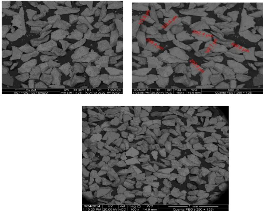
**Fig. 2 : Scanning electron microscope of typical manganese ore samples (-250+125μm)**
