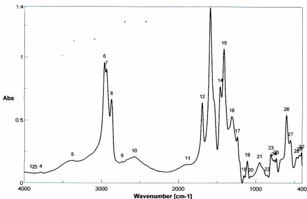
**Fig. 7 : Fourier transform infrared spectroscopy of Mn-2-ethyl hexanoat**
